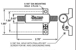
F FEMALE TO FEMALE WITH INTEGRAL BRACKET MODEL CX-FFFB
