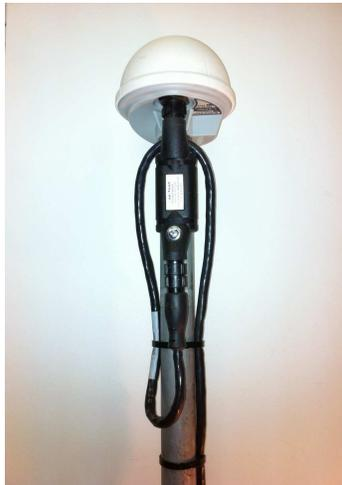
10. Secure all cables with cable ties and to pay attention to drip loops and cable strain considerations.
